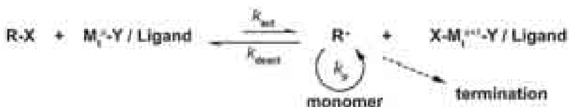
Figure 4 The mechanism of transition metal-catalyzed ATRP. M_t represents a transition metal, R represents the polymer chain, X represents a halogen atom, and Y represents another ligand or the counter ion. k_p is the polymerization rate, k_{act} and k_{dact} are the activation and deactivation constants [165].
