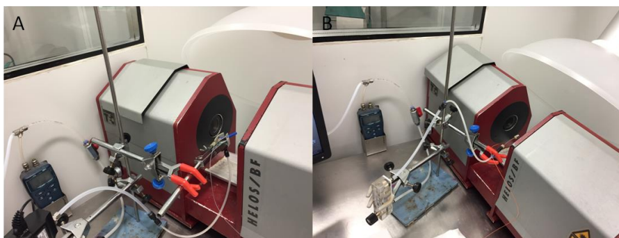
Figure 4.4. Pictures of the Sympatec Helos/BF Magic laser diffraction system used for the assessment of aerosols' droplets size measurements carried out at Ingeniatics Tecnológicas (Seville, Spain), using the FB240 (A) and FB100 (B) nozzles.
