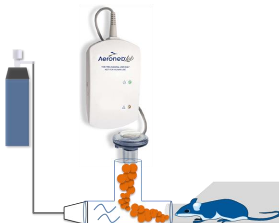
Figure 4.3. Illustration of the Aeroneb Lab Micropump Nebulizer connected to the rat holder.
