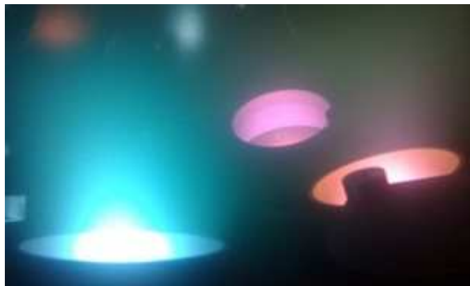
Figure 1.2. Plasma from UHV chamber of ATC 1800 UHV sputtering system (AJA International Inc, MA) induced in three magnetrons ejecting ions from titanium (blue plasma), gold (orange plasma) and silicon (pink plasma) targets under 24 sccm of argon flow.
