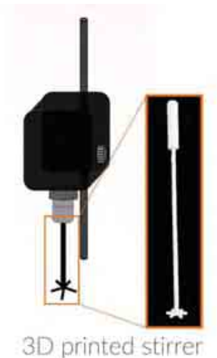
Figure 2.34. Polylactic acid (PLA) 3D printed stirrer that worked attached to a mechanical stirrer
