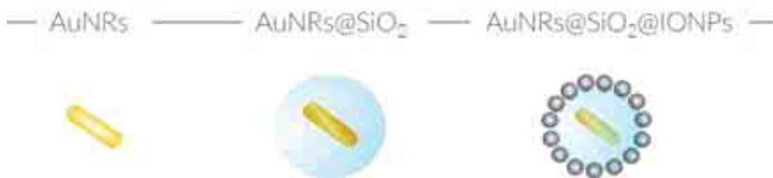
Figure 4.1. Schematic representation of the NPs obtained at each synthetic step. In this process, AuNRs were synthesized, covered by mesoporous silica (AuNR@SiO 2 ) and IONPs were finally grown onto the silica shell to obtain AuNR@SiO 2 @IONPs.
