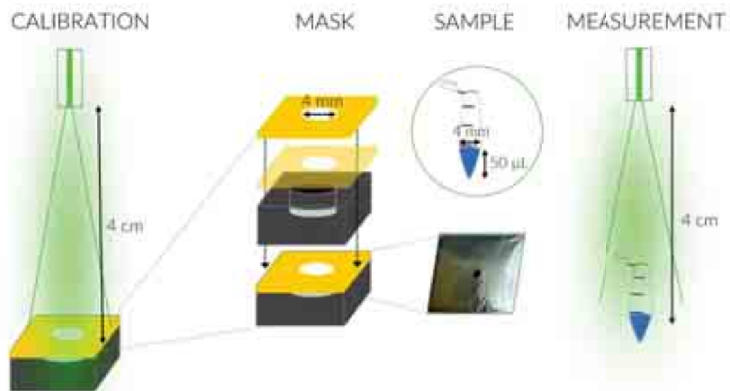
Figure 5.3. Scheme of the set-up for the calibration and irradiation of samples when measuring with a non-collimated beam or a collimated beam with a spot size bigger than the irradiation area.
