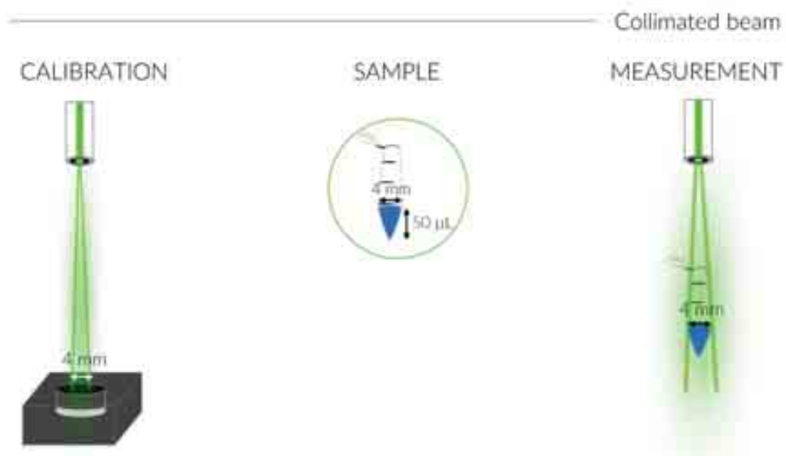
Figure 5.6. Schematic representation of the laser configuration when calibrating and measuring using a collimator with a beam spot size of equal area as the irradiation area.
