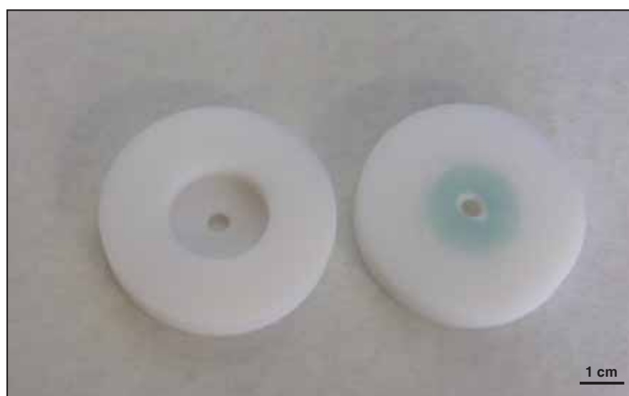
Figure 6.16: Teflon holder for RICM experiments. Left: top view. Right: bottom view. The glass coverslip is fixed up-side down with two-component dental glue to the bottom of the holder.
