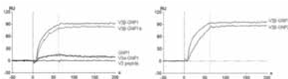
Figure 21. SPR experiments. mAb 447-52D was coupled to Proteon sensor chip using the recommended procedure until final 250 RU. A) Sensograms show the binding of V3 peptide (0.05 mg/ml) and GNP1, V3 \beta -GNP1, V3 \beta -GNP1b, V3 \alpha -GNP1 (0.2 mg/ml) to mAb 447-52D. B) Sensograms show the binding of V3 \beta -GNP1 and V3 \beta -GNP1b (0.2 mg/mL) to mAb 447-52D.
