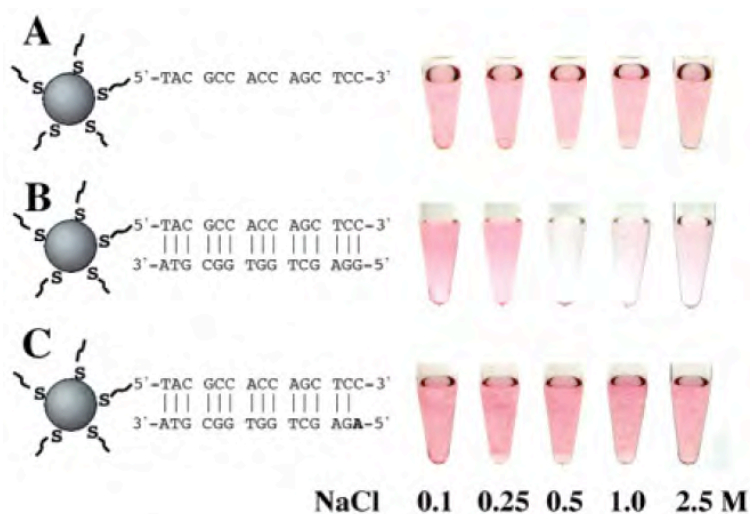
Figure 1.23. Aggregation behavior of DNA-AuNPs at various NaCl concentrations, at room temperature: (A) without a target DNA, (B) with the complementary target, and (C) with a target containing a single base mismatch at its 5' terminus. The final concentrations of the particle, the probe DNA, and the targets were 2.3, 500, and 500 nM, respectively. Adapted from 116 .
