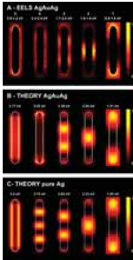
Figure IV.10. A: spatial distribution of plasmon modes for a short silver-gold-silver nanowire ( AgEn = 0.5 ) as measured by EELS; the numbers refer to the same modes as in the vis-NIR spectrum of Figure IV.9A . B: BEM simulations of EELS maps associated to the plasmon modes shown in A , for a nanowire containing the pentatwinned gold nanorod core. C: Simulations for a silver nanowire with the same dimensions. The simulated maps are normalized to the maximum intensity in each case. The silver (gold) surface is indicated with solid (broken) white lines in the calculated maps.
