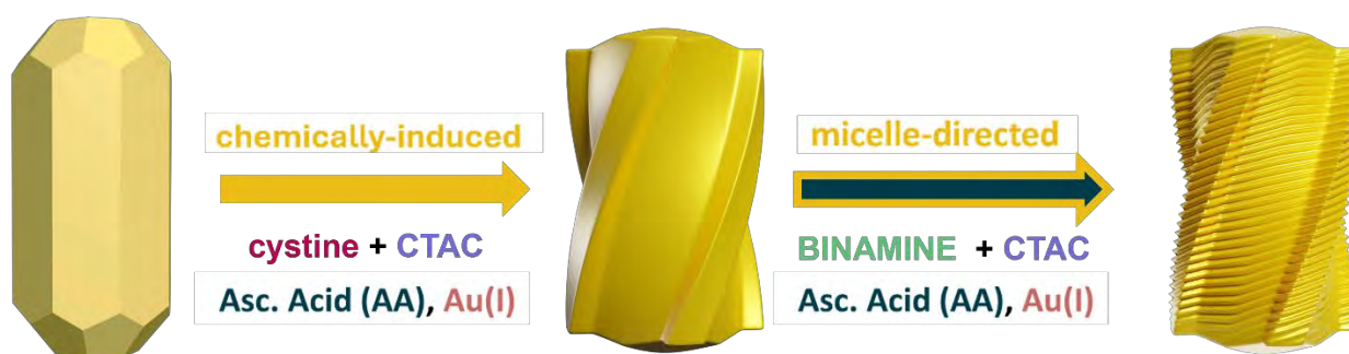
Figure 5.9. Schematic of general approach to form “double-chirality” products. Starting achiral gold nanorods are first subjected to the chemically-induced chiral growth mechanism, using cystine to produce chiral products with a smooth twisted morphology. These products are then isolated and subjected to a subsequent micelle-directed chiral reaction mediated by BINAMINE, forming helical wrinkles in a “shell” that surround the smooth chiral “core”.
