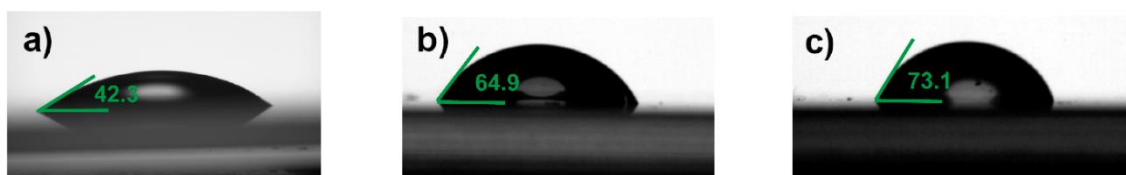
Figure 153. Contact angles of a) ITO-coated glass treated with piranha solution, b) ITO/G c) ITO/G-(3,4-(C 18 H 37 O) 2 Ph).
