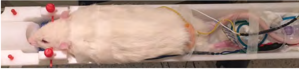
Figure 1.14: Animal laying on its belly in sphinx position in a MRI-compatible 'bed'. On the left, the nose cone for gaseous anaesthesia is visible. The cables on the right are for measuring the rectal temperature; the blues lines are connected to a pressure sensor (under the animal's chest) to monitor the respiration rate. The animal's head can be fixated with the red ear-bars on the left.
