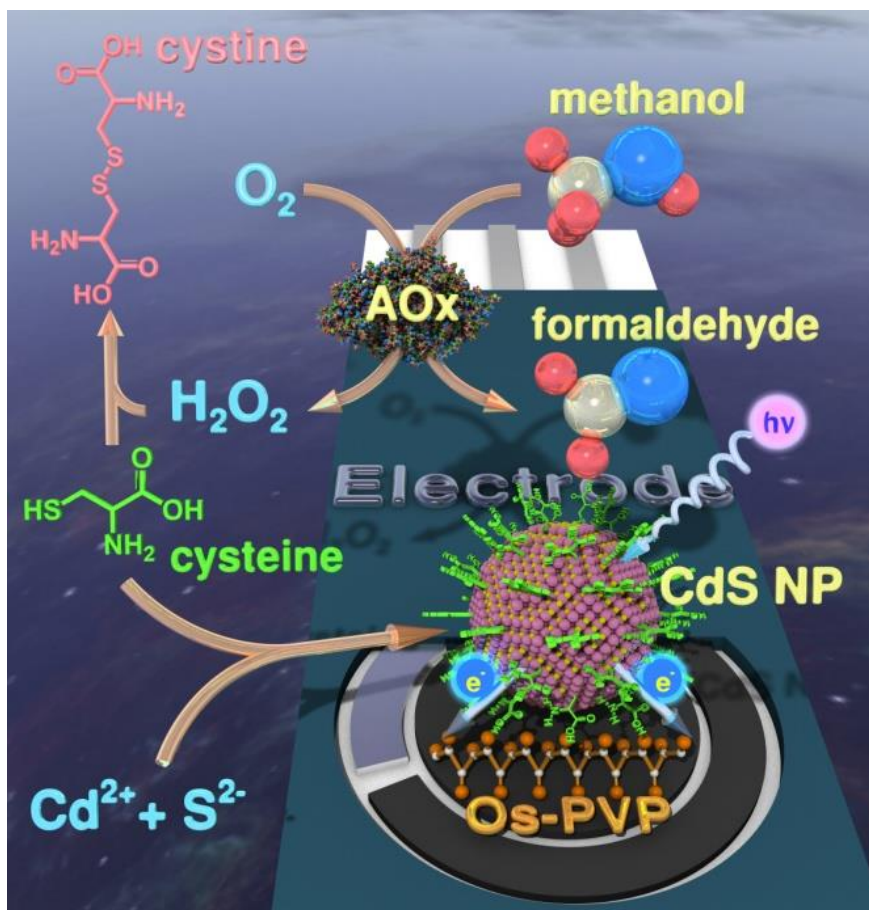
Scheme 2. Photoelectrochemical assay for methanol through detection of CdS QDs “wired” by an Os-PVP complex to the surface of a screen-printed carbon electrode.
