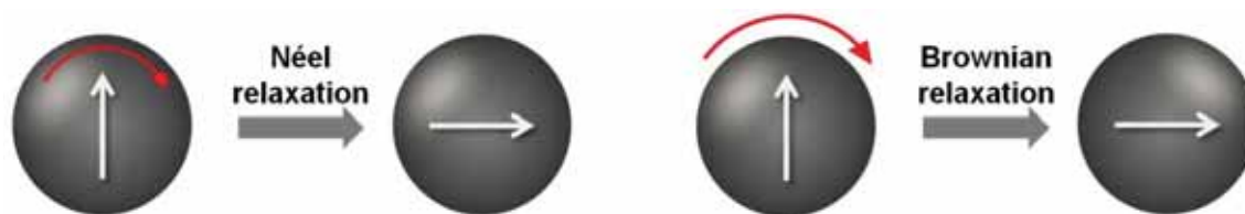
Figure 29. Heating dissipation processes of IONPs under an AMF. Néel relaxation is related to the alignment and relaxation of the spins while the Brownian relaxation is determined by the rotational mobility of the nanoparticles.
