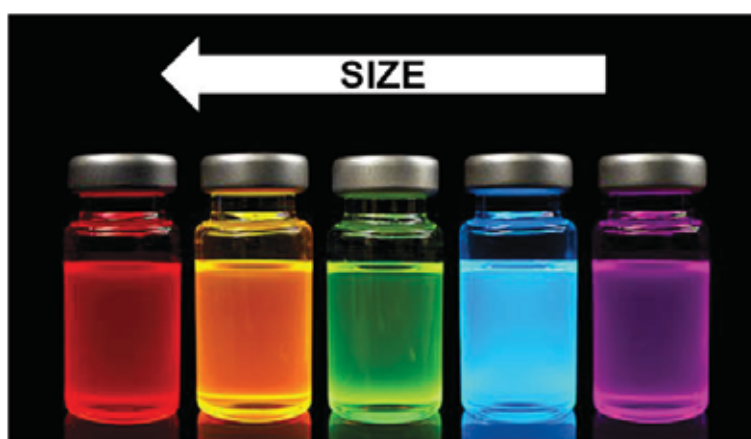
Figure 13. Size dependent fluorescent emission of semiconductor nanocrystals, quantum dots.
